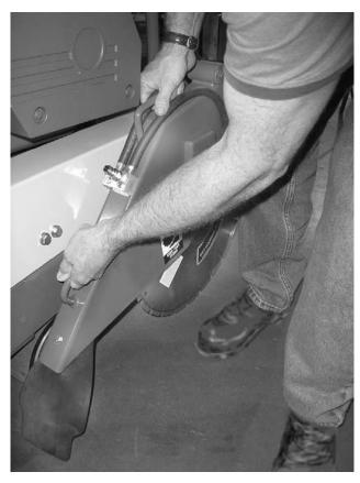
Figure 16. Removing The Blade Guard
